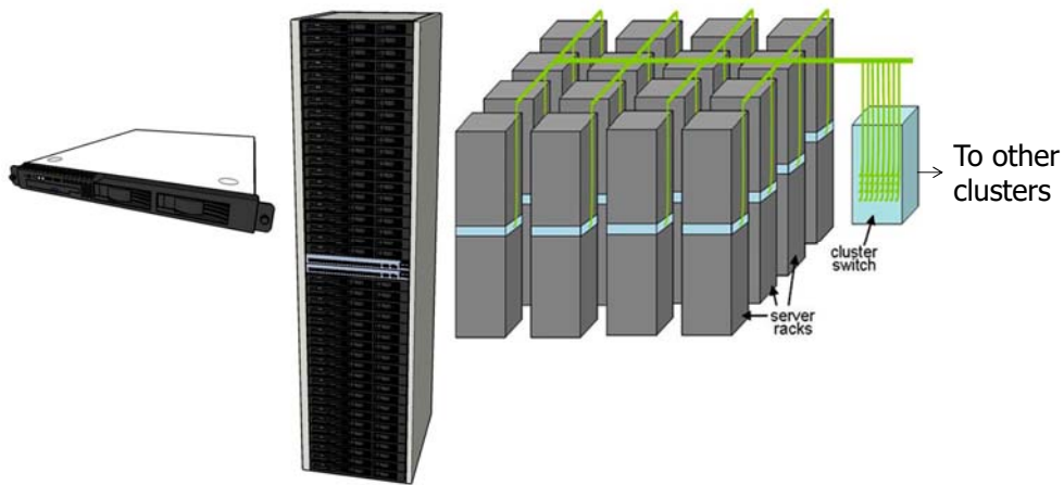
Figure 1.1: Sketch of the typical elements in warehouse-scale systems: 1U server (left), 7' rack with Ethernet switch (middle), and diagram of a small cluster with a cluster-level Ethernet switch/router (right).
