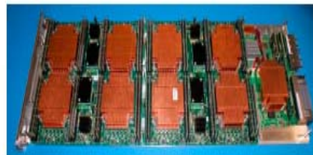
Figure 1. A Cascade blade which consists of 8 Xeon sockets, organized as 4 dual-socket nodes, and a single Aries ASIC.
