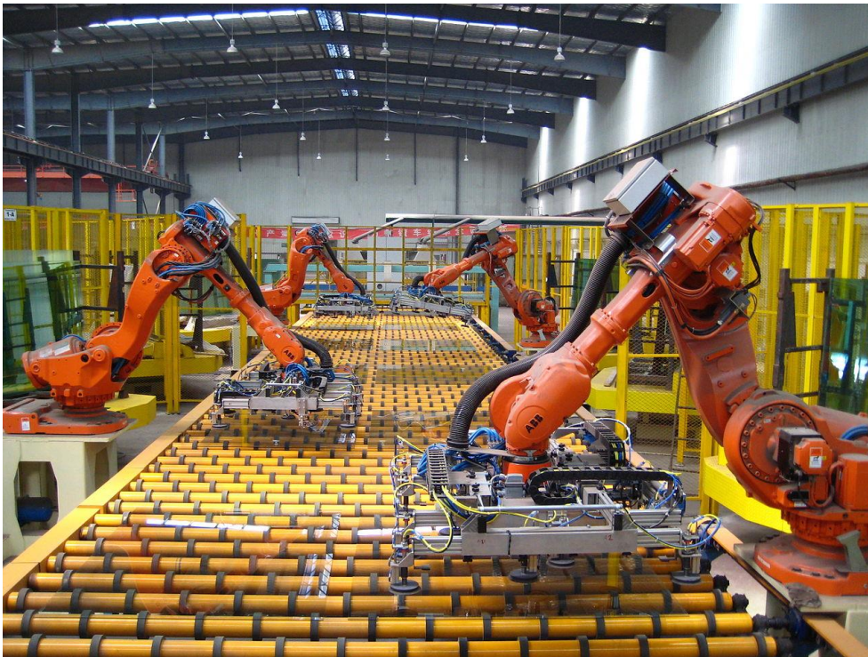
Robotized Float Glass Unloading. ICAPlants
