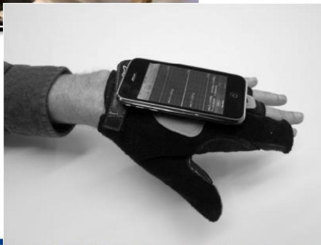
Fig. 1. iPhone wireless accelerometer application for characterizing Parkinson's disease tremor.
